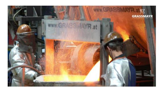
One of the highlights and a very exciting moment in the production process of bells is the casting itself. With a temperature of ca. 1.100 ° C, the liquid bronze flows into the clay forms.
